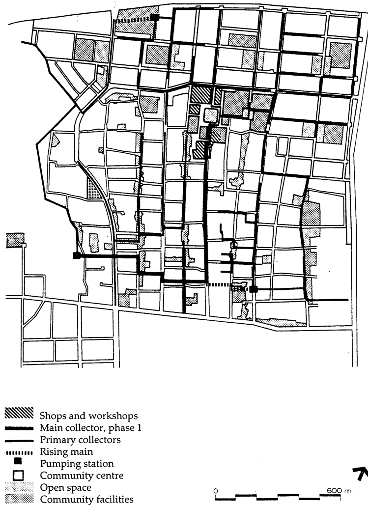
Figure 5.5 Hai El Salaam sewerage Source: Arab Republic of Egypt, 1978: vol. 1
